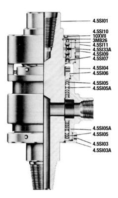
These swivels are manufactured and designed to fill a need when conventional swivels are not practical or applicable. Side inlet swivels find a wide application when using hydraulic, top-head drive rigs. Mounted below the hydraulic assembly, they prevent contamination of hydraulic fluid caused by leakage in conventional swivels. Auger rigs can be converted to circulating, rotary drilling rigs.
