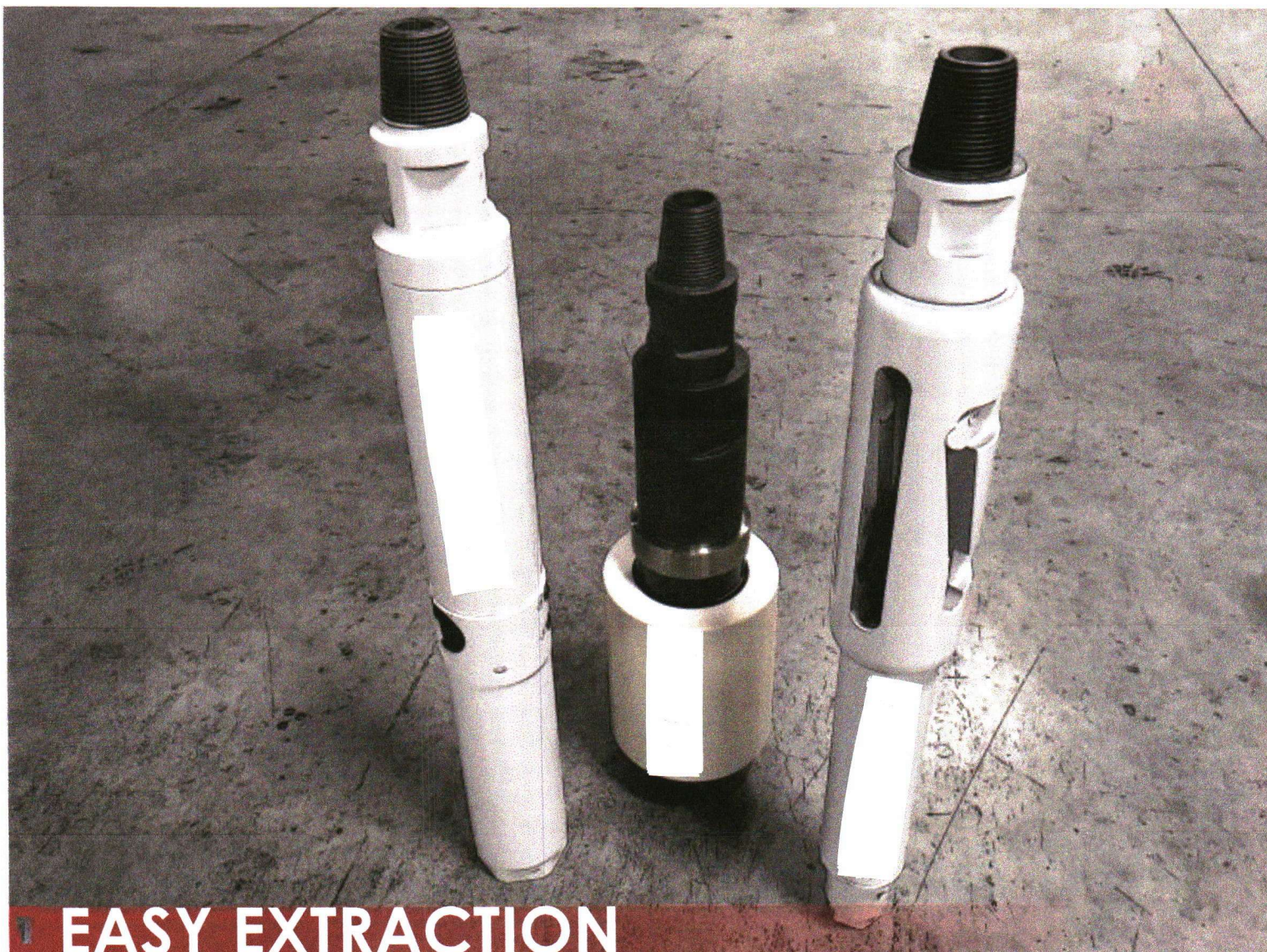
Left: 6" Casing Cutter, Middle: 200 lb Extractor hammer, Right: 6" Casing Perforator
