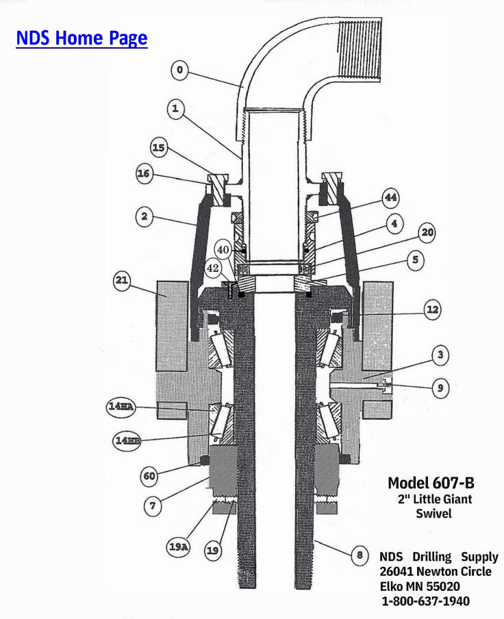
Item (4) has left hand thread Item (44) has left hand thread Item (2) has right hand thread Item (0) has right hand thread both ends Item (8) has left hand thread at bottom and right hand thread for item(7) Item (7) has right hand thread and adjusts bearings
