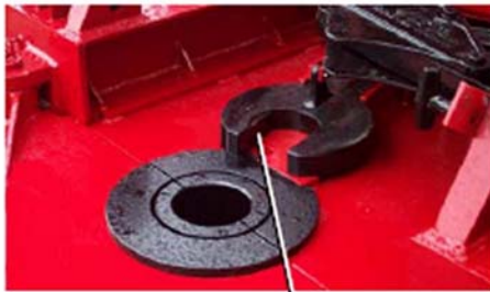
ALIGN FLATS WITH SLIDING FORK WRENCH (TABLE WRENCH)
