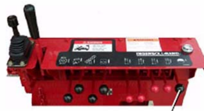
WATER INJECTION CONTROLS
