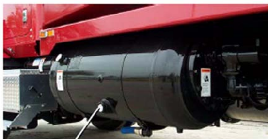
COMPRESSOR OIL LEVEL GAUGE
