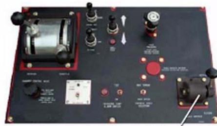
PULL TABLE WRENCH CONTROL TOWARD OPERATOR TO EXTEND THE SLIDING FORK WRENCH
