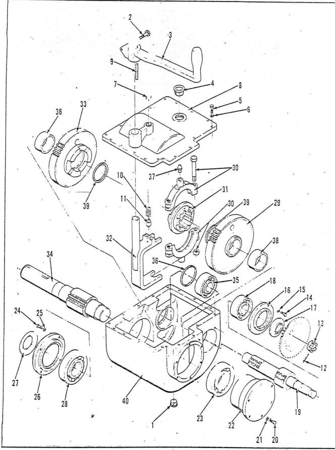
Figure 3-45. Pulldown Transmission
