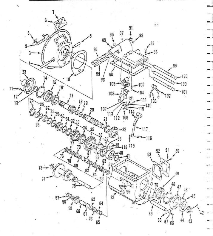
Figure 3-37. Rotary Table Transmission
