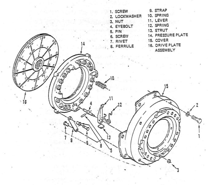
Figure 3-35. Rotary Table Clutch 180
