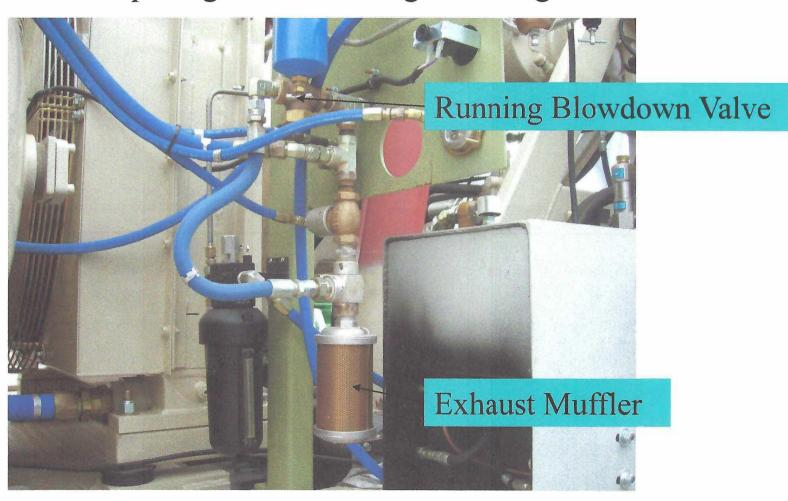
If the inlet cylinder is stroked shut and the blowdown valve is open and pressure continues to increase it may be necessary to adjust the butterfly inlet valve.
