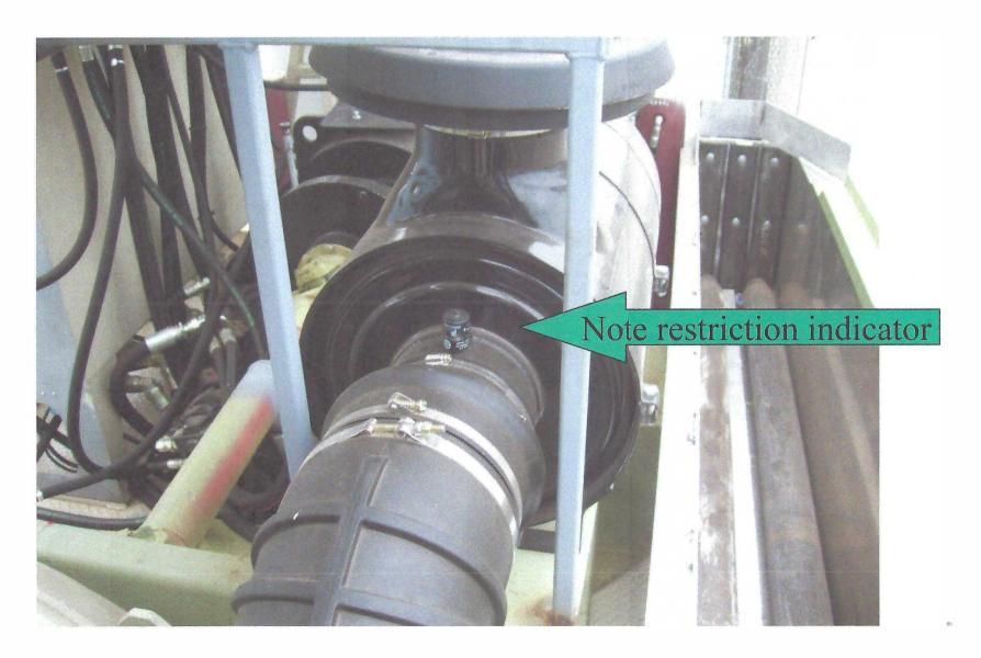
There should be a filter indicator located on the filter housing. Filters should also be visually inspected. There is a inner and outer filter. Many times the inner filter will have a colored eye that will show restriction. Do not blow out filters and try to re-use. Filters can be contaminated by compressor oil due to emergency or high speed shut-downs.
