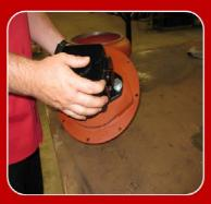
• Hold Motor & Impeller together while flipping over till the Impeller side is on the work surface.
