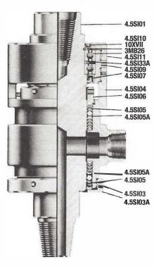
These swivels are manufactured and designed to fill a need when conventional swivels are not practical or applicable. Side inlet swivels find a wide application when using hydraulic, top-head drive rigs. Mounted below the hydraulic assembly, they prevent contamination of hydraulic fluid caused by leakage in conventional swivels. Auger rigs can be converted to circulating, rotary drilling rigs.
