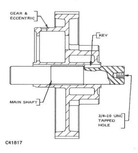
FIGURE 9 - ECCENTRIC AND MAIN SHAFT ASSEMBLY
