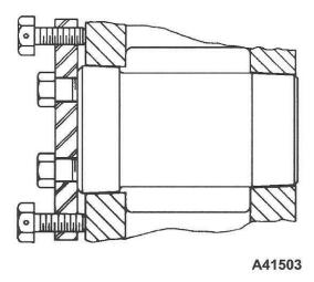
FIGURE 10 - CROSSHEAD PIN REMOVAL-FXX, FXD & FXE
