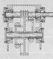
The **Failing** Model FM-45 is a duplex reciprocating type power slush pump designed for maximum volume without sacrifice of working pressure and compactness.
