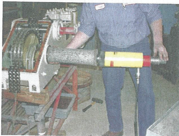
FIGURE 13: Preparing to pull the eccentric sprocket shaft.
