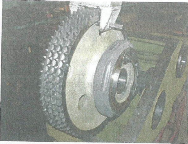
FIGURE 13: After the eccentric shaft is removed, the eccentric sprocket, connecting rods and crosshead assembly may be removed from the main frame.
