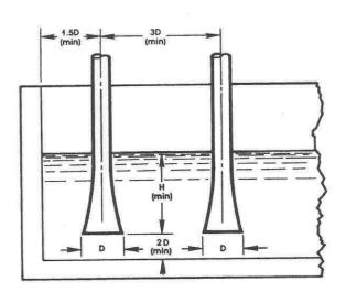
This can be used as a guide for minimum submergence and piping design.
