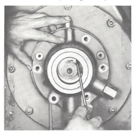
Figure 29 — Installing Connecting Rod
