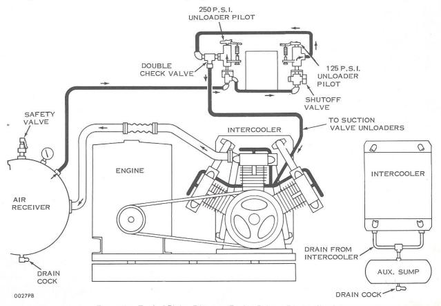
Figure 4 — Typical Piping Diagram (Engine Driven) Rig Application
