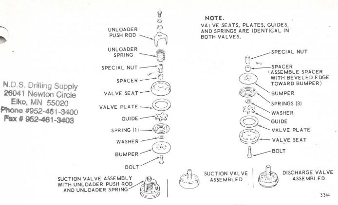
Figure 13 — Suction and Discharge Valves
