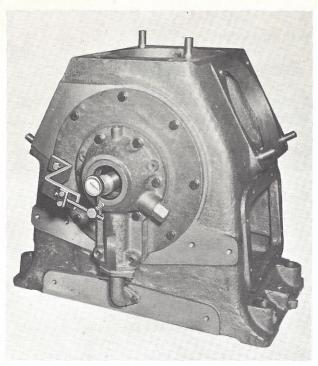
Figure 33 — Checking Crankshaft End Thrust
