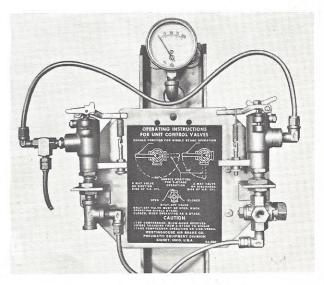
Figure 3 — Pressure Control System
