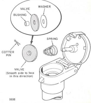
Figure 26 — Oil Filler Tube Breather Cap
