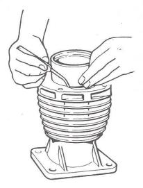
Figure 24 — Checking End Clearance
