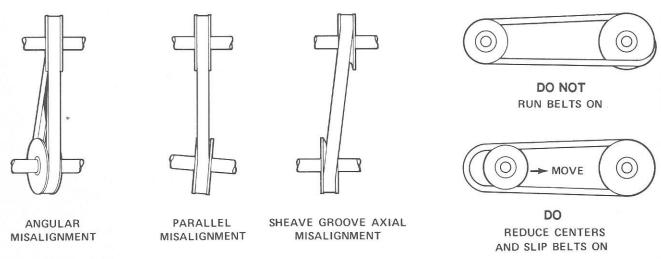
Shafts must be in angular and parallel alignment and the sheave grooves axially aligned to obtain proper performance of V-belt drives. Angular alignment is obtained by levelling shafts.
