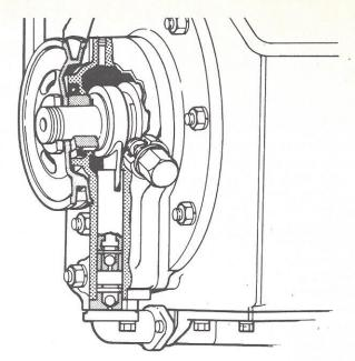
Figure 2 — Lubricating Oil Pump
