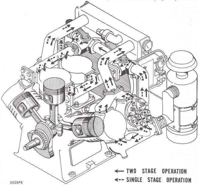
Figure 1 — Schematic Diagram of Air Flow Thru Compressor
