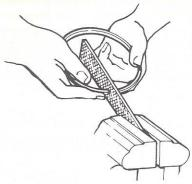
Figure 21 — Filing Piston Ring Gap
