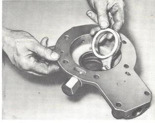
Figure 28 — Removing or Installing Plunger
