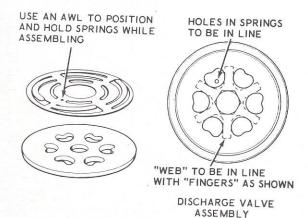
Figure 16 - Valve Reassembly
