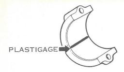
PLASTIGAGE INSERTED ON BEARING SHELL BEFORE IT HAS BEEN REINSTALLED AND TIGHTENED
