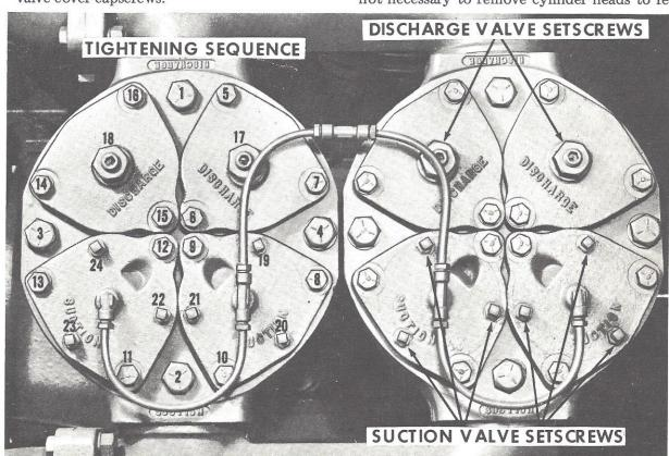
Figure 17 - Cylinder Head Tightening Sequence and Location of Setscrews
