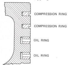
Figure 22 — Piston Ring Installation
