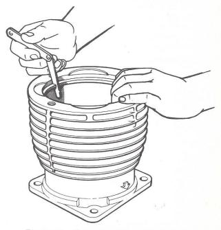
Figure 20 — Checking Ring Gap End Clearance
