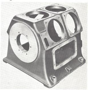
Figure 31 - Compressor Crankcase
