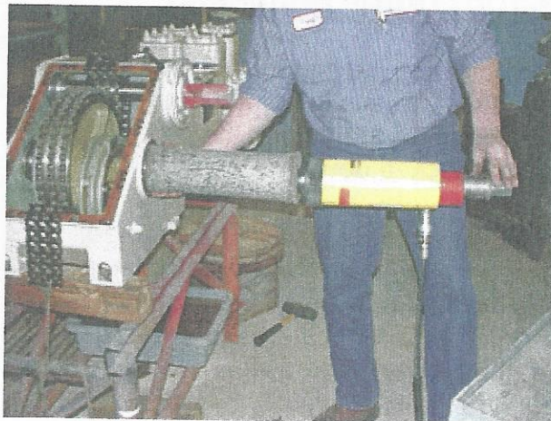
FIGURE 13: Preparing to pull the eccentric sprocket shaft.
