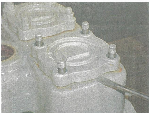
FIGURE 1: Removing the valve cover.
