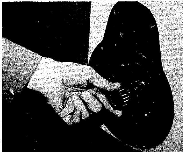
19. Install needle roller bearings into output shaft.
