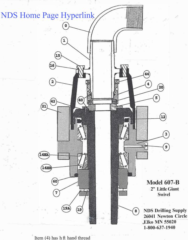
Item (4) has left hand thread Item (2) has right hand thread Item (0) has right hand thread both ends Item (8) has left hand thread at bottom and right hand thread for item(7) Item (7) has right hand thread and adjusts bearings
